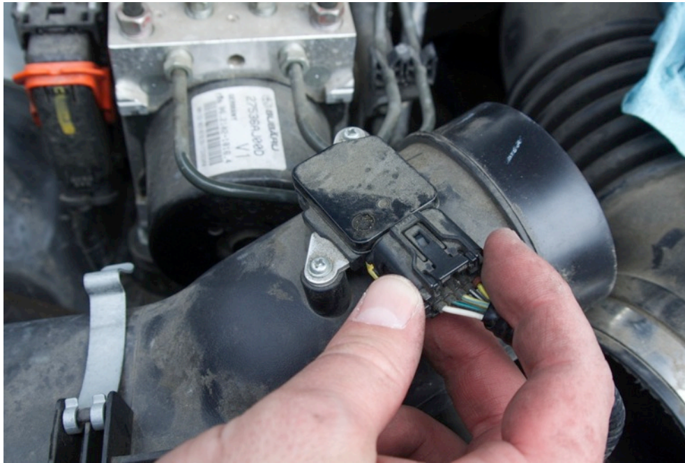
Figure 30: Reattach Mass Air Flow Sensor Wire
