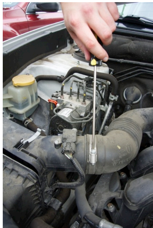
Figure 9: Loosen the Air Box Hose Clamp
