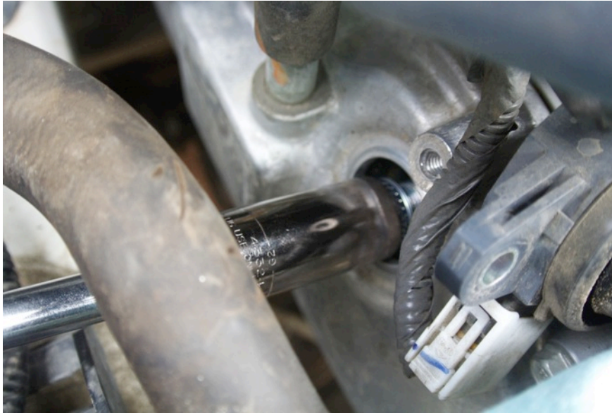
Figure 26: Insert the New Spark Plug
