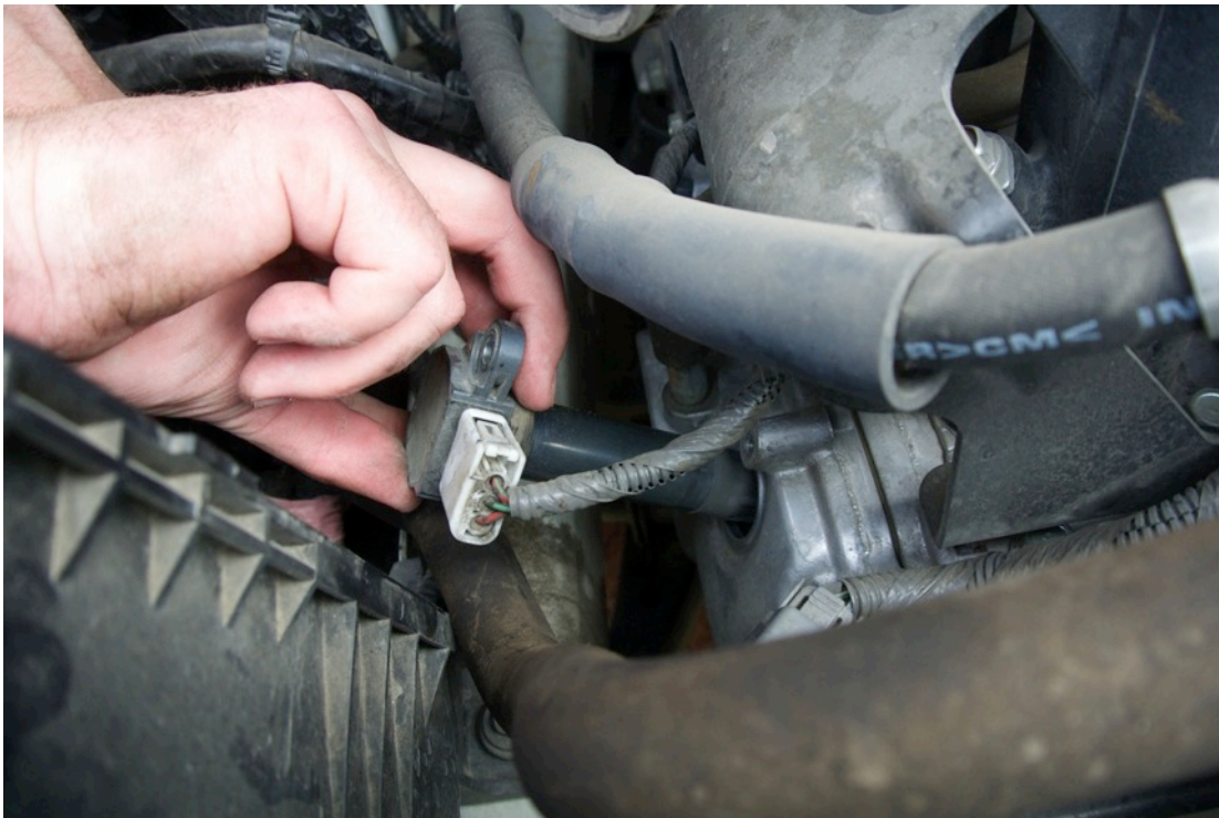
Figure 21: Pull The Coil From the Engine
