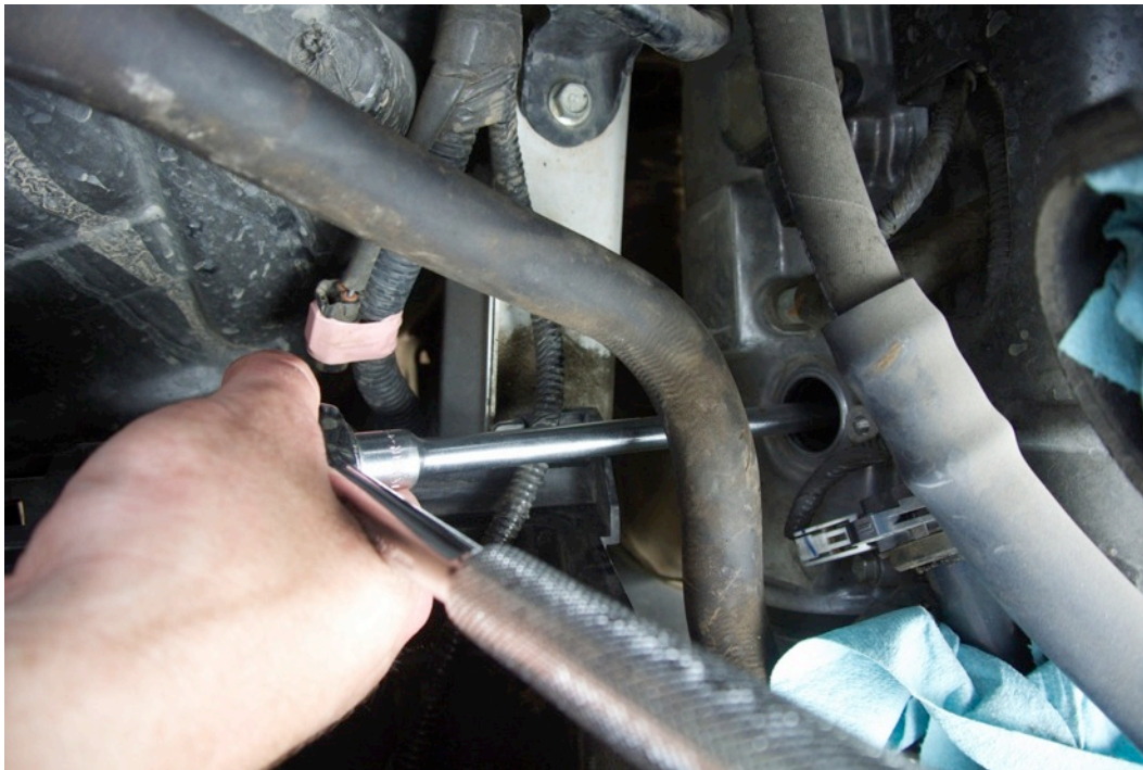
Figure 23: Insert the Spark Plug Socket into Opening
