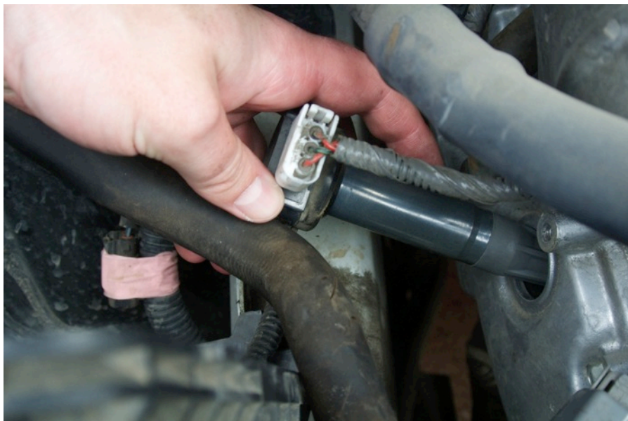
Figure 27: Insert the Spark Plug Coil
