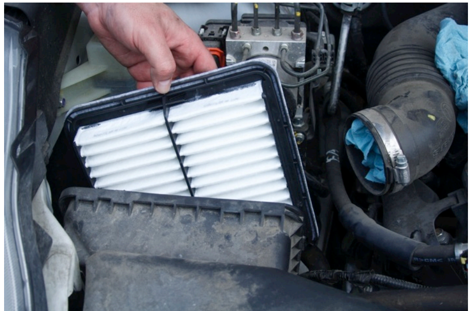
Figure 29: Insert Air Filter
