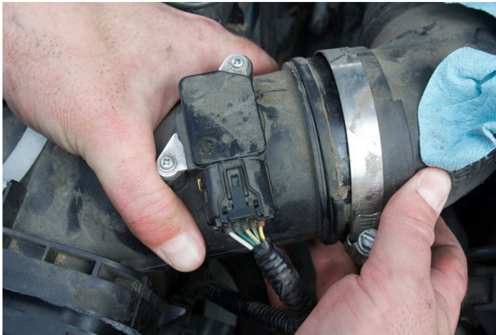
Figure 31: Reattach Air Box to Hose
