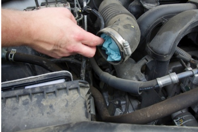
Figure 9: (Optional) Plug the Air Box Hose
