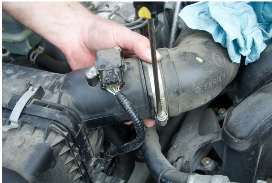
Figure 33: Tighten Air Box Hose Clamp
