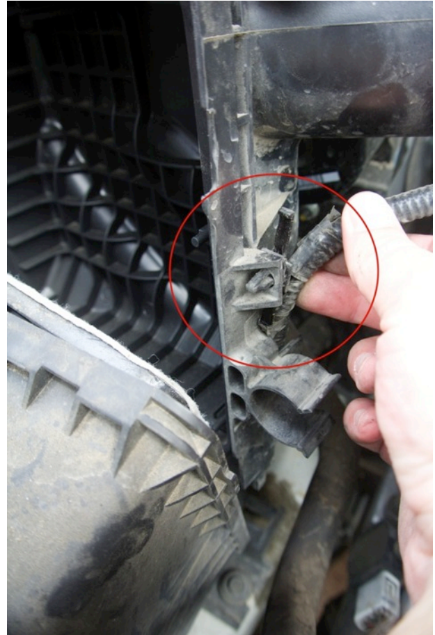
Figure 12: Remove Mass Air Flow Sensor Wire Out Of Bracket
