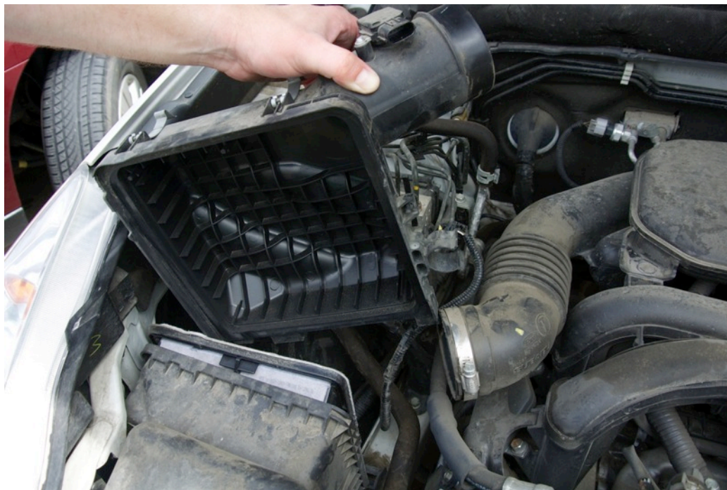
Figure 13: Remove Air Box Front Half From Engine Bay
