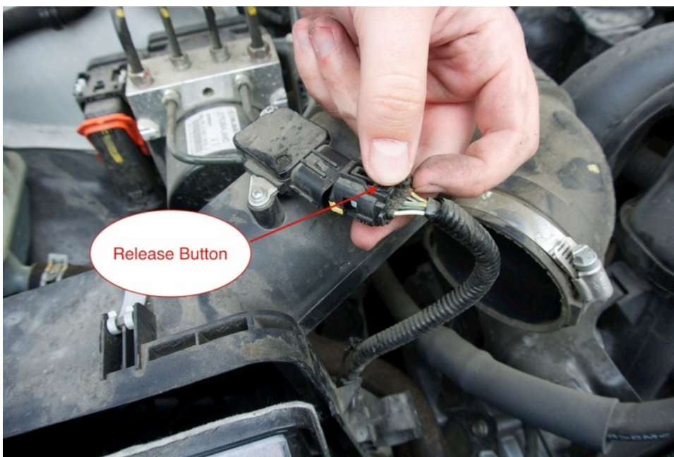
Figure 11: Disconnect Mass Air Flow Wire
