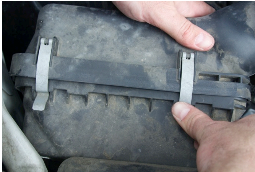
Figure 32: Closed Air Box Latches
