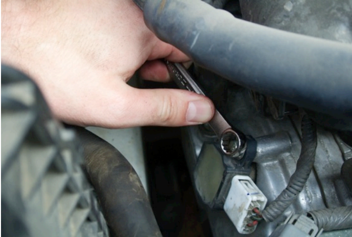
Figure 28: Replace Bolt on Spark Plug Coil
