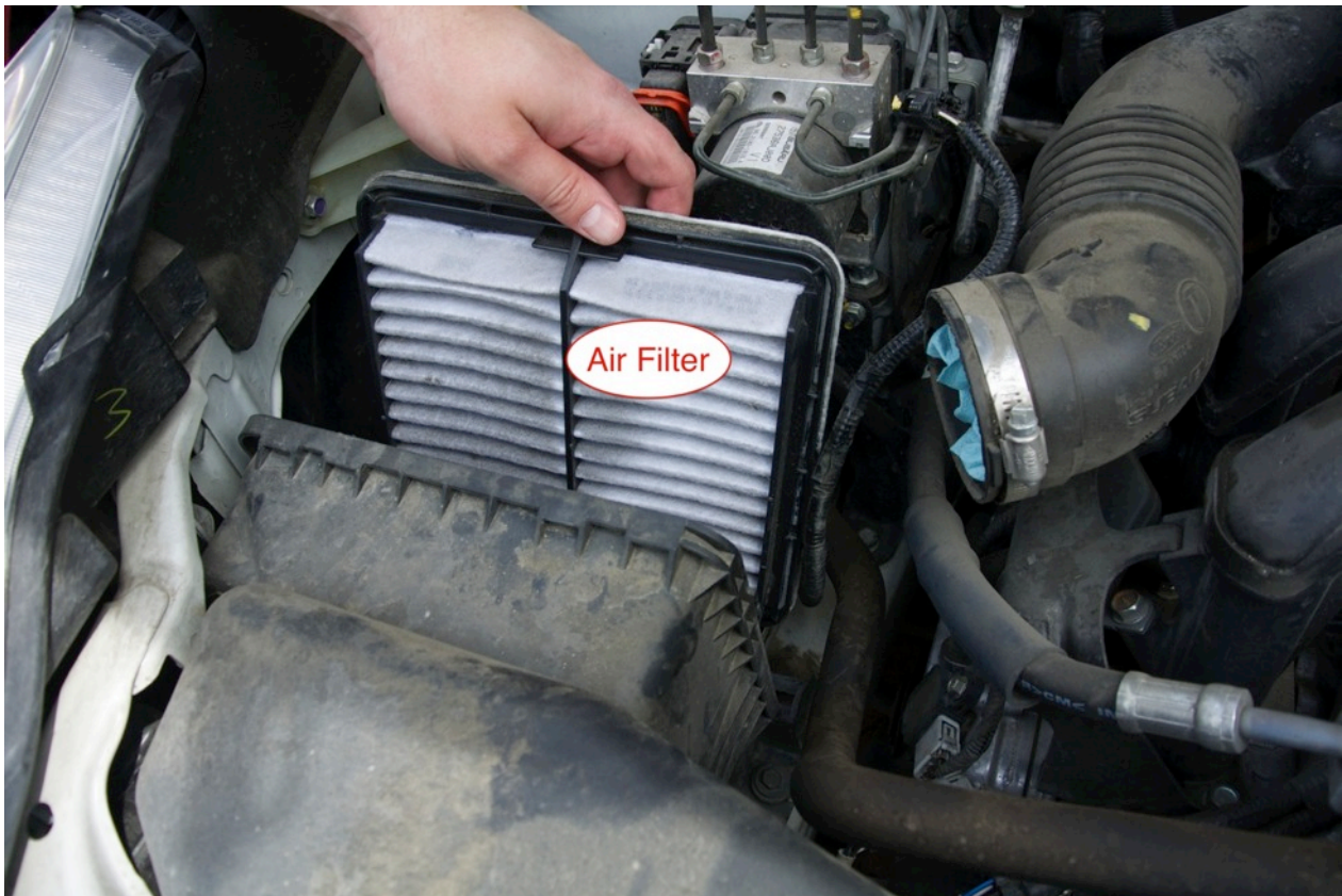
Figure 10: Remove the Air Filter
