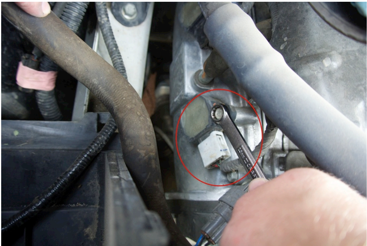
Figure 14: Remove Bolt on Spark Plug Coil
