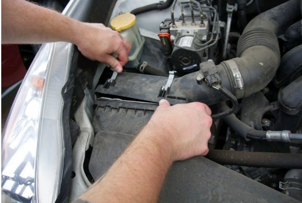
Figure 8: Disconnected Air Box Latches
