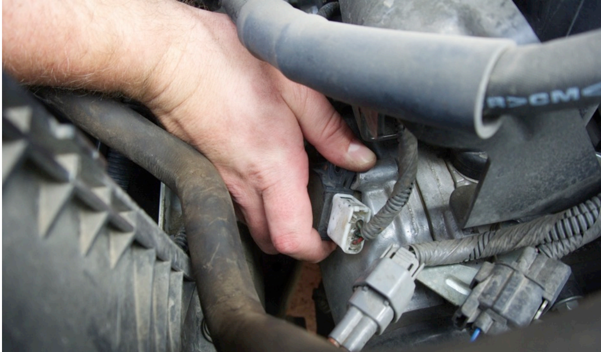
Figure 20: Gently Twist the Coil
